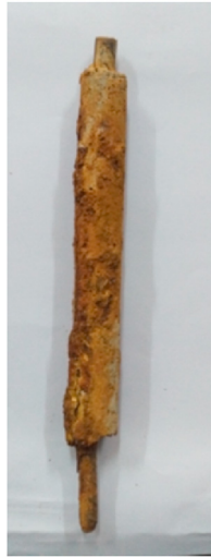
Fig. 13. The 7-d cured RCCP at the end of the 5th day of EK treatment process (Sadeghian et al., 2021).
