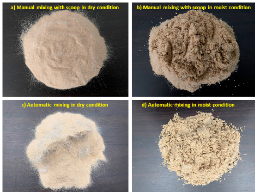
Fig. 4. Sand–fiber admixture after the mixing process performed by four different methods.
