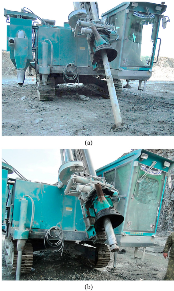
Fig. 8. DTH hammers: (a) COP64.2 and (b) PV170 M.
