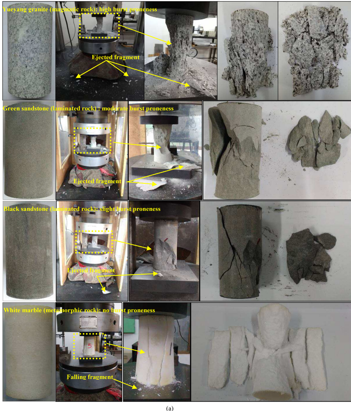
Fig. 3. Typical rock specimens used for deriving the LES and LED laws: (a) Specimens before and after testing, and (b) Bursting scenarios of specimens (Gong et al., 2018b).
