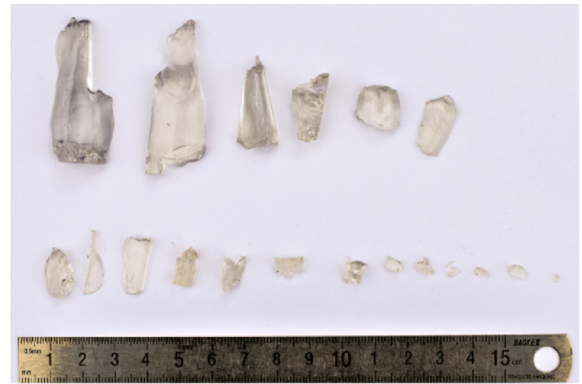
Fig. 4. The broken 3DP specimen at -45 °C after UCS test.
