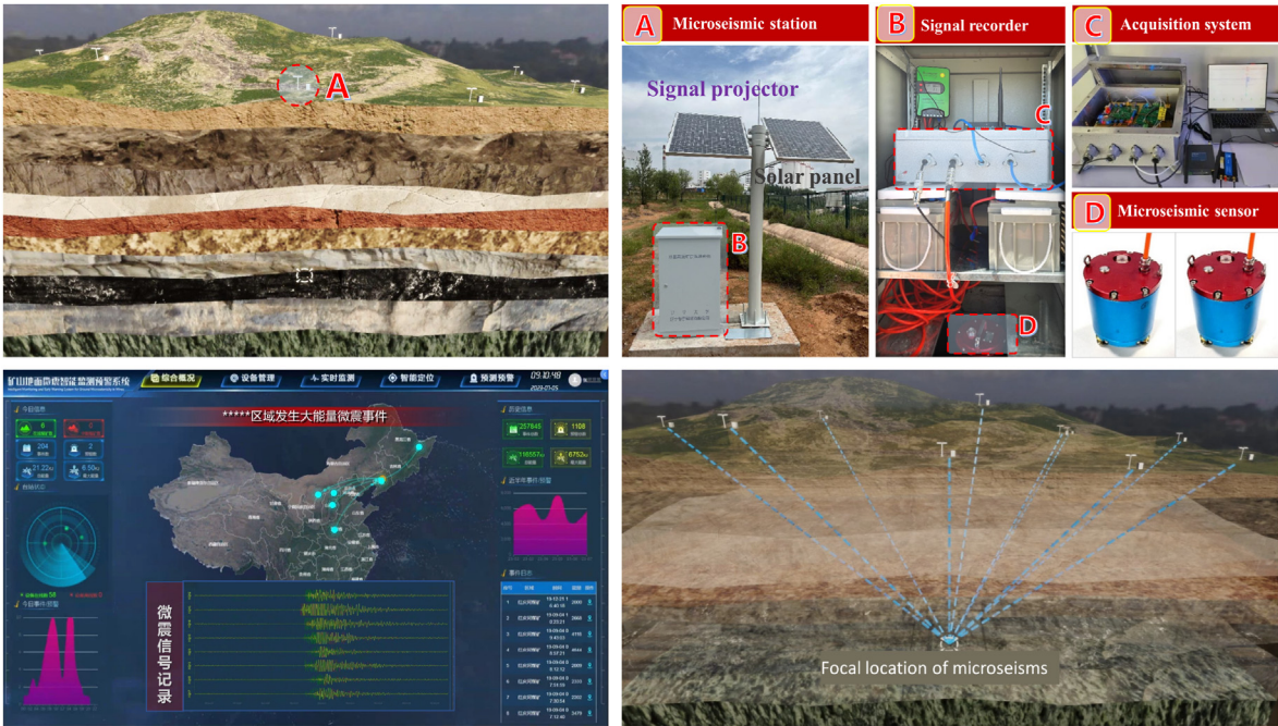
Fig. 28. Monitoring and early warning system for coalburst control in China.
