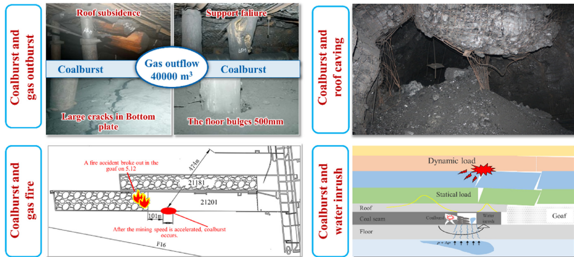
Fig. 8. Combination of coalbursts and other disasters.
