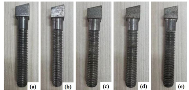
Fig. 13. The modelled scrapers with various metal materials: (a) 45#, (b) 06Cr19Ni10, (c) 42CrMo4, (d) 40CrNiMoA, and (e) WC-Co.
