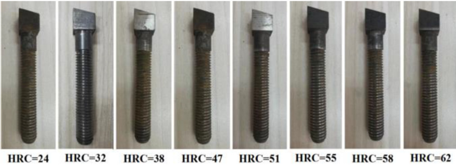
Fig. 17. The modelled scrapers with Rockwell hardness (HRC) values of 24, 32, 38, 47, 51, 55, 58 and 62.
