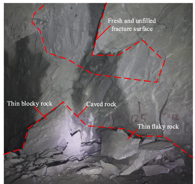
Fig. 16. Rock mass failure at the junction area between the shaft and the second gallery.
