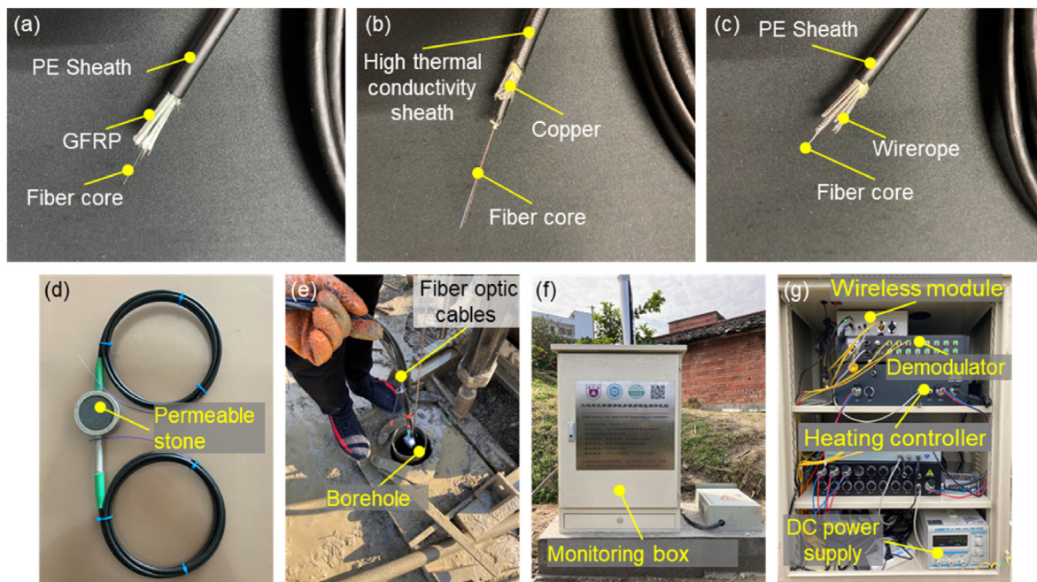
Fig. 4. Field installation of UWFBG sensing arrays: (a) Temperature sensing cable; (b) Moisture sensing cable; (c) Strain sensing cable; (d) Pore water pressure cell; (e) Instrumented borehole to be downwards placed and backfilled; (f) Monitoring box at the top of the borehole FOS3; and (g) In situ interrogator.
