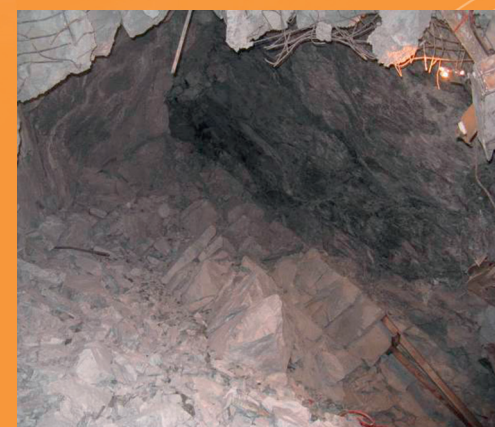
An example of tectonic burst in a deep tunnel of the Jinping II project (C. Zhang et al.)
