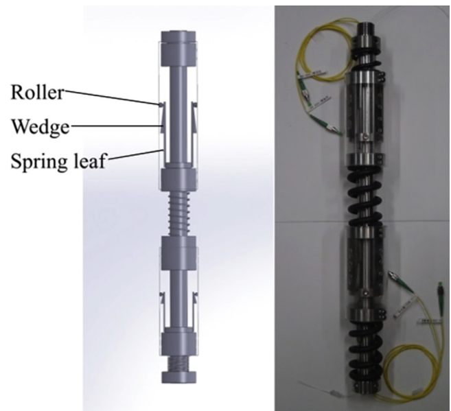
Fig. 6. The FBG extensometer.
