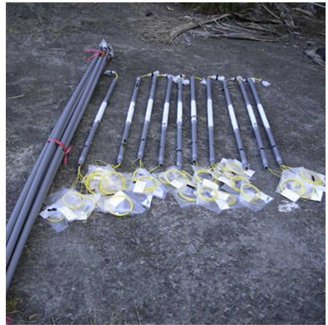
(b) The packaged FBG sensor array.
