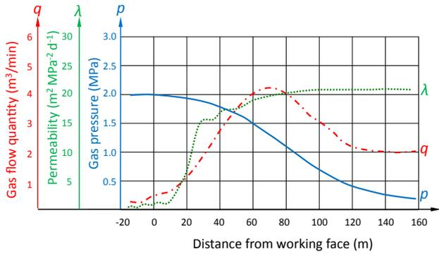
Fig. 8. The performance of gas drainage from de-stressed seams.
