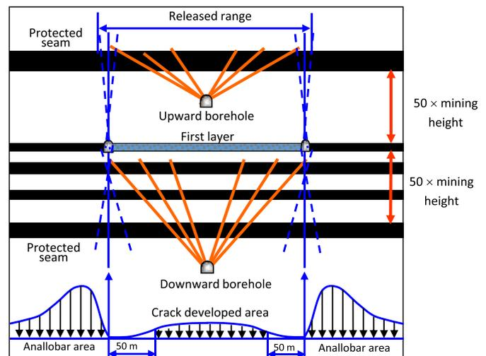
**Fig. 7.** The principle of gas drainage from de-stressed seams.
