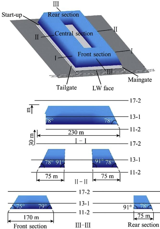
Fig. 4. An annular-shaped overlying zone. “LW face” means longwall face.
