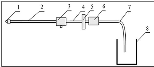
1-drill bit; 2-compound drill pipe; 3-side-in rotary connector; 4-end-drill pipe; 5-drill chuck; 6-normal incidence rotary connector; 7-sampling hose; 8-sample container
