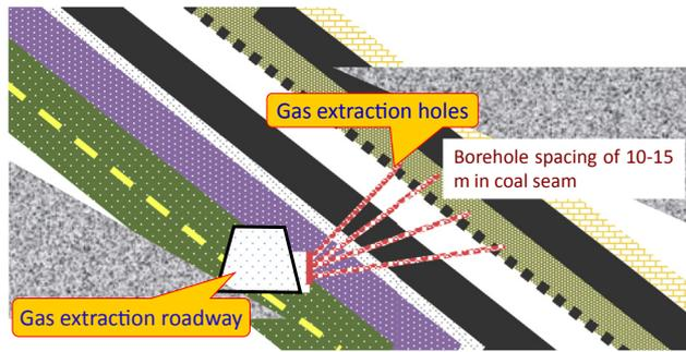
(a) Cross measure gas drainage from a main gas tunnel.
