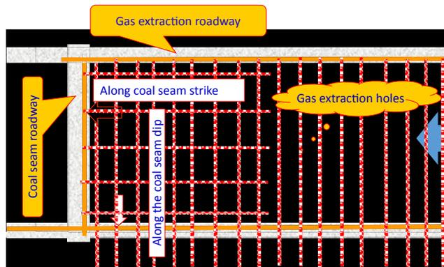
(c) Inseam gas drainage from a main gas tunnel.
