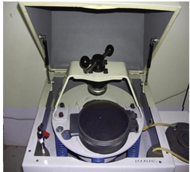
Fig. 13. A coal sample crusher in gas content measurement system.
