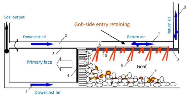
Fig. 2. Integrated pillarless coal mining and gas drainage with Y-type ventilation. Number 1 is panel air intake, 2 is secondary air intake, 3 is filled sidewall, 4 is longwall face, 5 is gas drainage pipelines, 6 is roof gas drainage boreholes along the face, 7 is panel air return, 8 is main air return, 9 is goaf, and 10 is floor gas drainage boreholes along the face.
