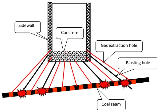
Fig. 15. Outburst prevention in coal uncovering in shaft sinking.
