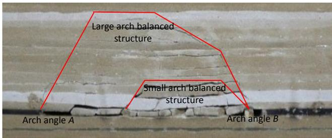
Fig. 5. The “arch in arch” structure and fan-shaped gas-rich zone.
