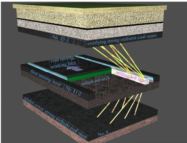
Fig. 9. Integrated pillarless coal mining and gas drainage with Y-type ventilation.
