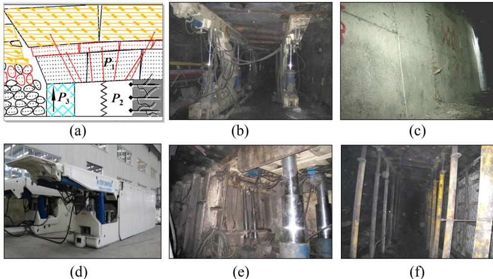
Fig. 10. Strata control with integrated pillarless coal mining and gas drainage. (a) Trinity surrounding rock control technology, (b) Auto mobile assistant enhanced bracket (P<sub>2</sub>), (c) Wall filling (P<sub>3</sub>), (d) Side formwork bracket for roadside filling, (e) Near template bracket for roadside filling, and (f) Roadway maintenance effect of underground level -900 m.
