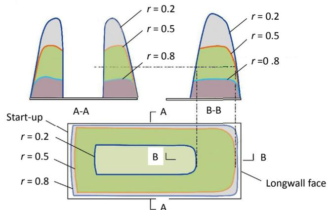
Fig. 3. A conceptual model of the stress reduction ratio.
