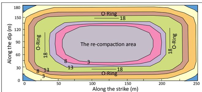
Fig. 1. O-ring fracture distribution and gas flow channels. The stress of mined-out area is given in the form of contour lines (unit: MPa).
