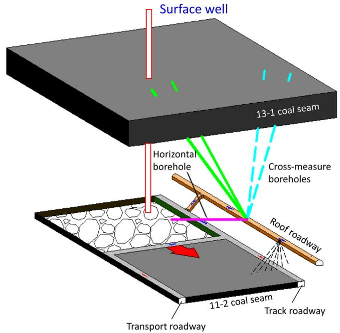
Fig. 12. An integrated approach of both surface and underground gas drainage.
