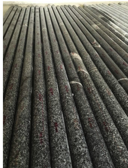
Fig. 12. (a) RQD classification showing the proportion of different rock mass qualities for four vertical boreholes (BS06, BS28, BS32 and BS33) at the Xinchang URL site; and (b) Intact 63-mm-diameter drilled cores extracted from borehole BS32.
