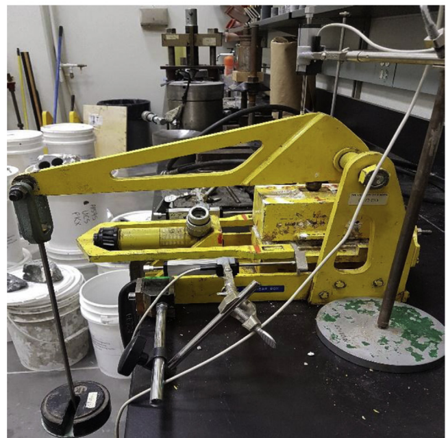
Fig. 5. Direct shear machine: (a) schematic, and (b) actual direct shear apparatus.
