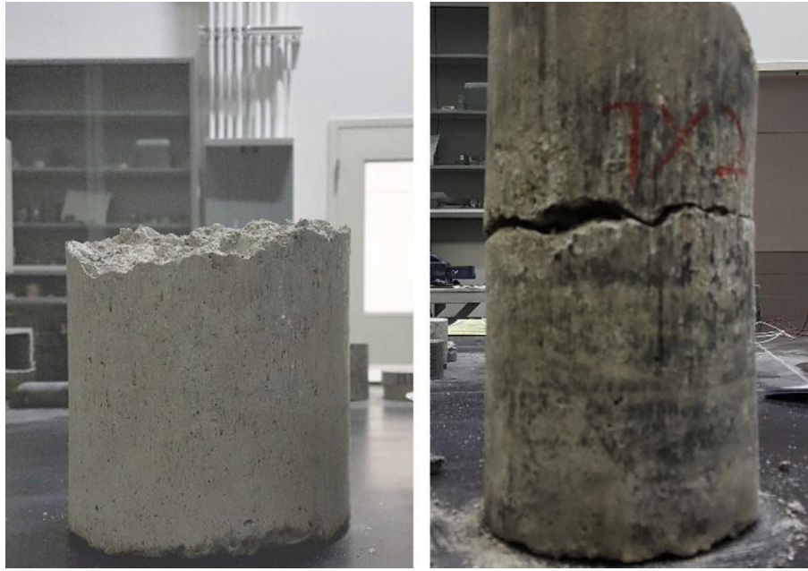
Fig. 8. Mode of failure of CRF under triaxial test.
