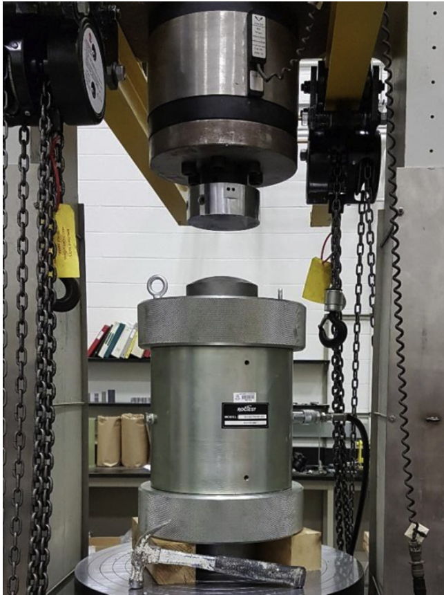
Fig. 4. The 154.2 mm diameter Hoek triaxial cell and 10,000 kN capacity loading frame INSTRON.
