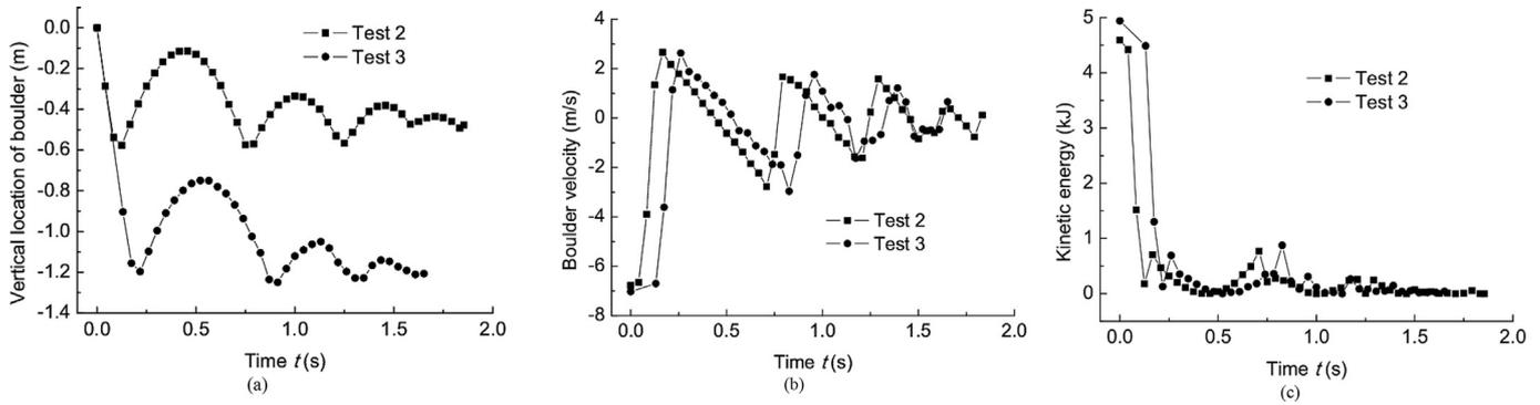
Fig. 9. Effect of the mesh length on mesh response: (a) Vertical trajectory, (b) Vertical velocity, and (c) Kinematic energy of the boulder in Tests 2 and 3.
