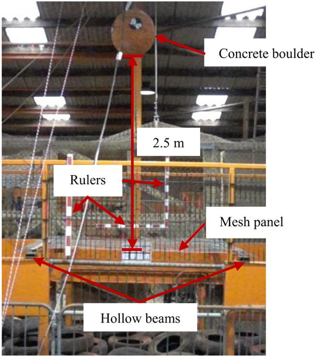
Fig. 5. Front view of Test 2.
