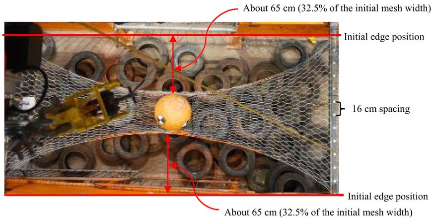
Fig. 10. Lateral deflection of the wire mesh of Test 3 (top view).
