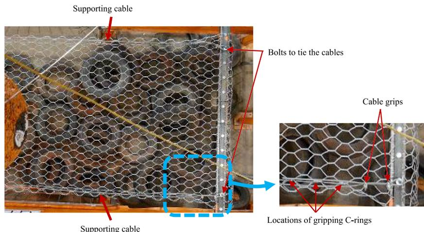
Fig. 4. Method for fixing supporting cables in the tests.
