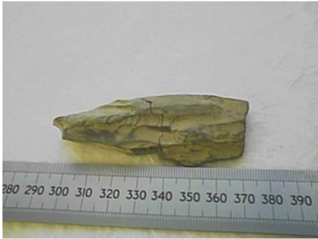
Fig. 3. Angular caving (Bradford et al., 2000).
