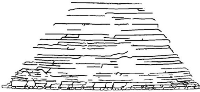
Fig. 7. Fracture field distribution based on similarity simulations (Wang et al., 2009).
