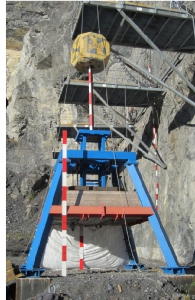
Fig. 17. The setup for the full-scale impact tests (Roth, 2014).
