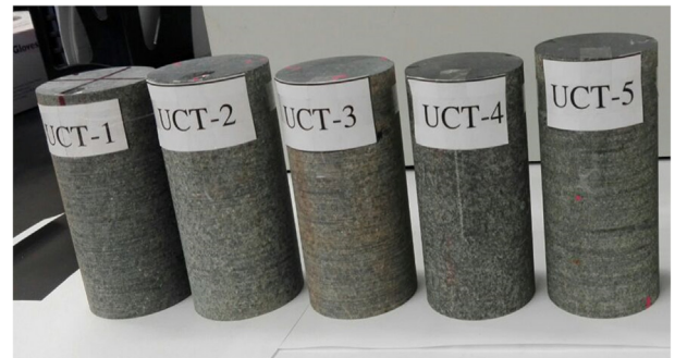
Fig. 2. Dolerite specimens prepared for the uniaxial compression tests.
