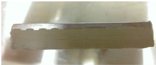
Fig. 15. Top half of sheared specimen with MLC showing no uneven vertical deformation after large-strain deformation.
