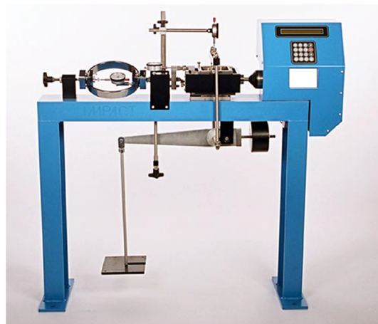
Fig. 1. Standard direct shear apparatus (Impact Test, 2021).
