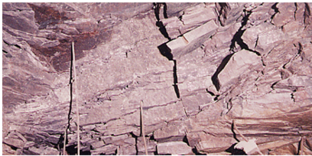
Fig. 11. Example of blocky ground created in the immediate vicinity of the excavation by stress-fracturing of a moderately jointed rock mass. Open fractures and shears illustrate the related bulking process due to geometric non-fit of blocks of hard rock.
