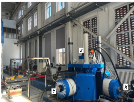
Fig. 10. True triaxial dynamic disturbance apparatus for deep hard rocks under high true triaxial stresses.
