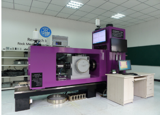
Fig. 3. True triaxial compression stress path testing apparatus for obtaining the complete stress-strain curve of deep hard rocks under high true triaxial stress paths (Feng et al., 2016a).
